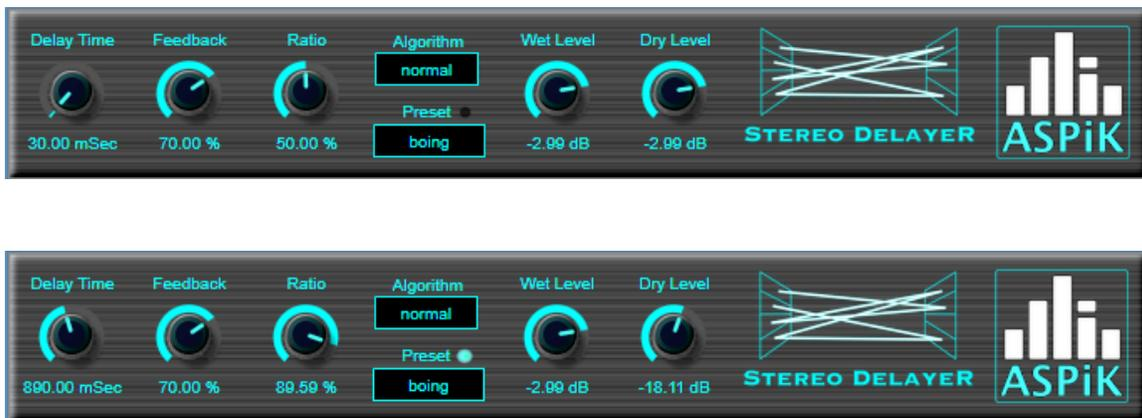
Figure A1.1: (top) a preset drop-list added to the ASPiK *StereoDelayer* project and (bottom) when the user moves any control, a “dirty GUI” LED lights up next to the “Preset” text, when the user selects a fresh preset, the LED turns off
