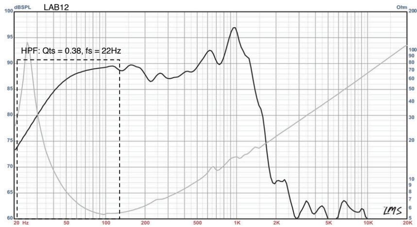
Figure 6.14: The Thiele-Small Parameters tell us immediately what the low-frequency cutoff and resonances are going to look like.
