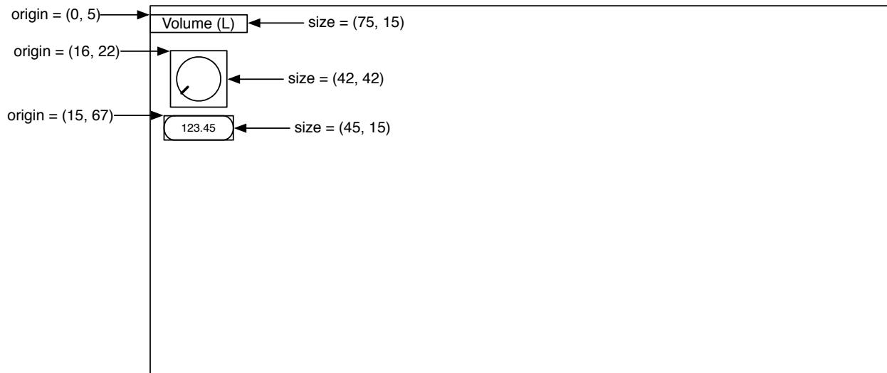
Notice that the coordinates of the origin values are relative to the ***frame***, whose upper left corner is (0, 0). This is the golden rule of VSTGUI object placement — the origin of the object is always relative to the origin of the parent container. So, we can now list our first three GUI objects that will need to be created and their origin/size values:
