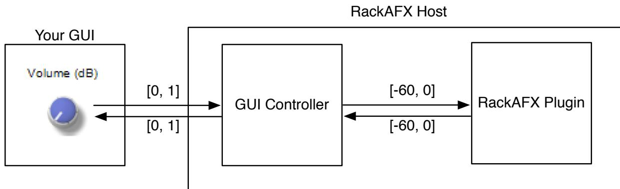
In this case, the GUI Controller object is part of the RackAFX host. For your custom GUI, the location of the object changes — your plugin now owns the GUI Controller object:
