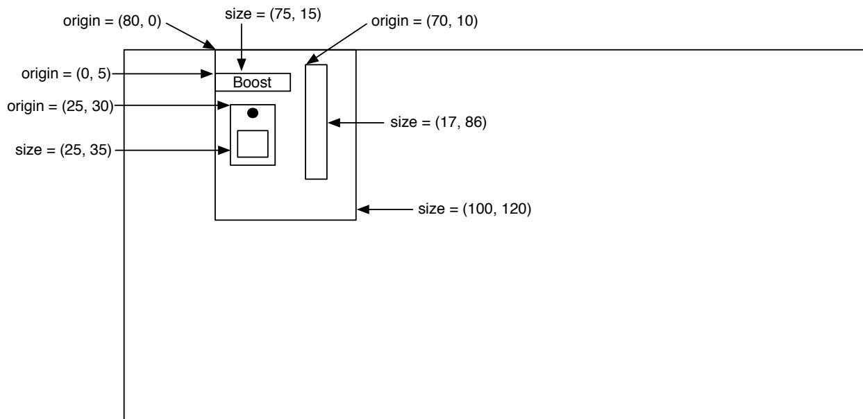
The inner view container's origin is relative to the frame's origin, however, the inner view container's sub-views are positioned relative to it's origin — for example the Boost label is (0, 5) where x = 0 is the left side of the inner view container. Now we can list the rest of the controls.
