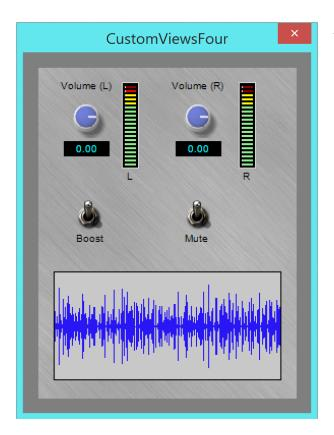
The custom *CView* object is at the bottom and displays the audio waveform.
