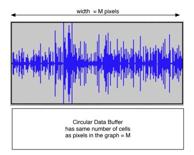
Here is the audio waveform view with the circular buffer below it and laying on its side. The trick to making this work is that the circular buffer has the exact same number of cells (memory locations) as the *CView* is wide, in pixels. When we plot the data, we will move one pixel at a time, drawing a line that represents the overall audio amplitude variable. Thus each cell in the buffer corresponds to one audio sample amplitude and that produces one line segment in the graph.
