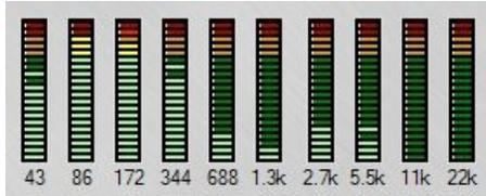
This Plug-In implements a simple spectrum analyzer by examining the 10 bins (a bin is an index number in the FFT array) of the FFT equally spaced across it and displaying their normalized values (0.0 to 1.0) on the LED Meters on the main GUI. The LEDs move according to the amplitudes of these bins. The FFT length (#defined as FFT\_LEN) is either 1024 or 2048 points. To get our nearly 10 octaves of audio, we find the bins for the 1024 point case as (Bin 0 is DC or 0 Hz):
